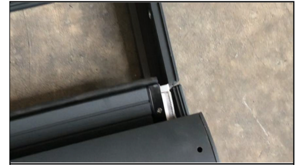
3. Put the rear rail into the end cover foot corresponding to the main body of the rolling curtain
