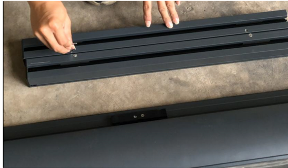
1. Unpack and use the hex wrench to disassemble the screws on the track
